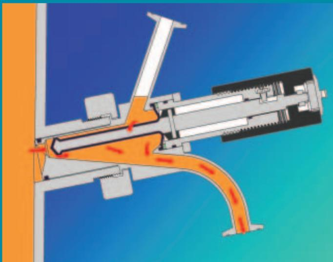
Valve open for sampling. Since all internal surfaces are smooth and declining, process material quickly flows down and out, even when installed in an inclined porthole.
