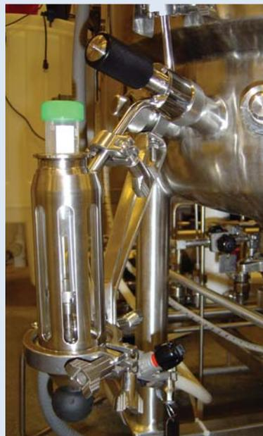
declining internal passages, is the only sampling valve on the market designed to sample through standard inclined 25mm sensor ports (Ingold, etc) for optimum draining and sample site flexibility.
